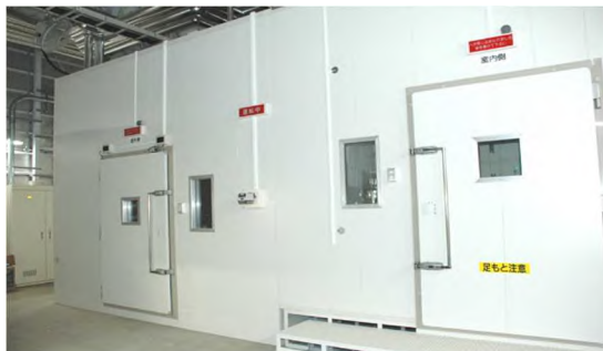
図③.2.1-1 Calorie meter, outdoor unit test room (left), and indoor unit test room
