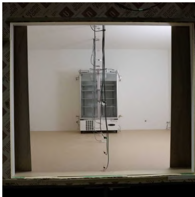
図④. 1.1-1 Model room for Leakage diffusion behavior examination of R290 (propane)
