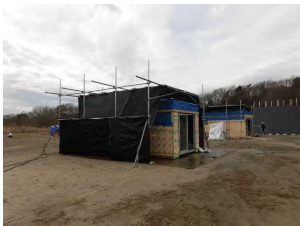
図③.2.1-1 Model room for Combustion effect evaluation of R290 (propane)
