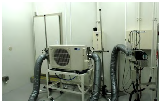
図③.2.1-2 Outdoor unit test room
