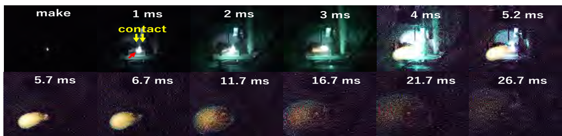
(b)7.0 vol% of R290、 resistive circuit、 700 W
