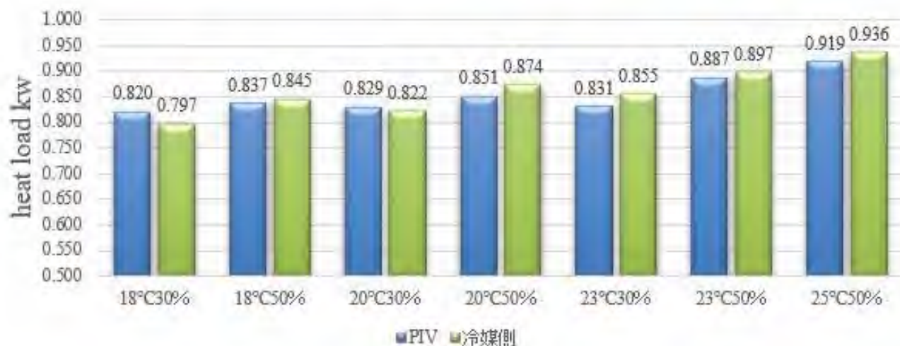
図②.3.3.5-7 Comparison of heat load test results by PIV and refrigerant flow measurement
