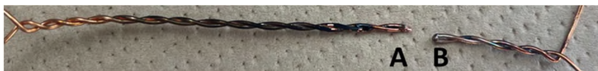
図②. 2. 2-36 Enameled wire after fusing
