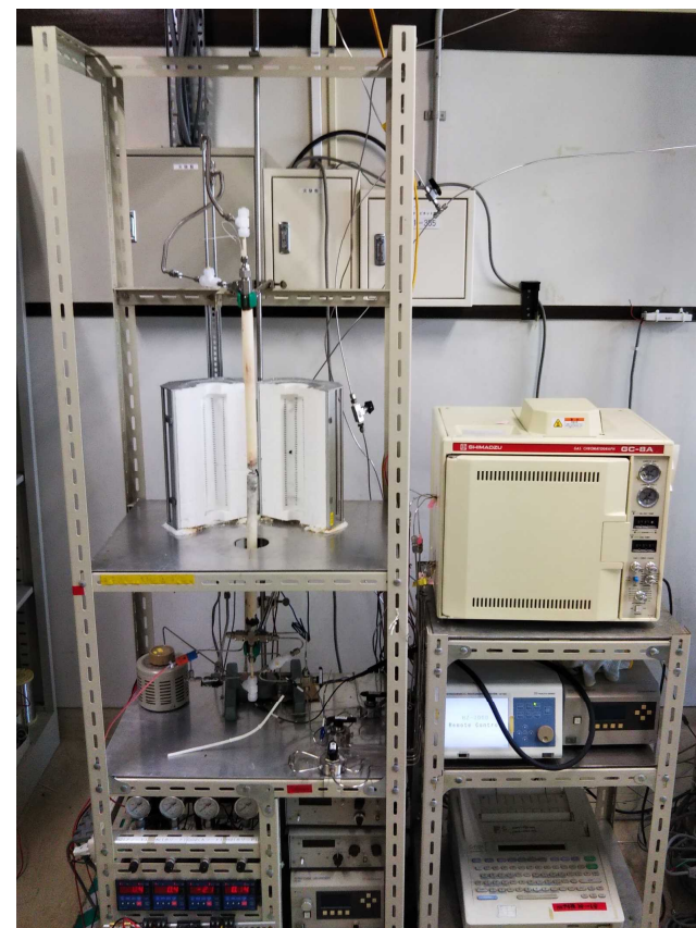
Fig. 1 Schematic diagrams and a picture of the CO 2 electrolysis system
