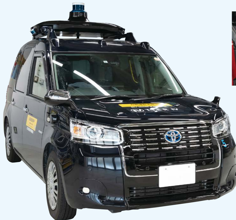
In addition to an Autoware controlled system, this experimental vehicle is equipped with 14 LiDAR devices and cameras, a global navigation satellite system, and an inertial measurement unit.
