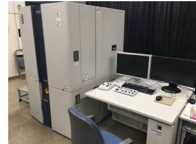
In-lens FE-SEM (Hitachi SU9000)
