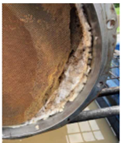
broken catalyst in NH 3 -SCR (by urea water)
