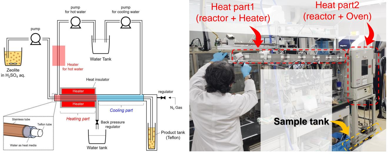
Machine for zeolite synthesis
