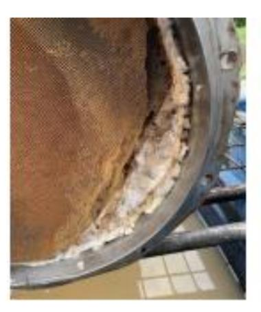
broken catalyst in NH<sub>3</sub>-SCR (by urea water)
