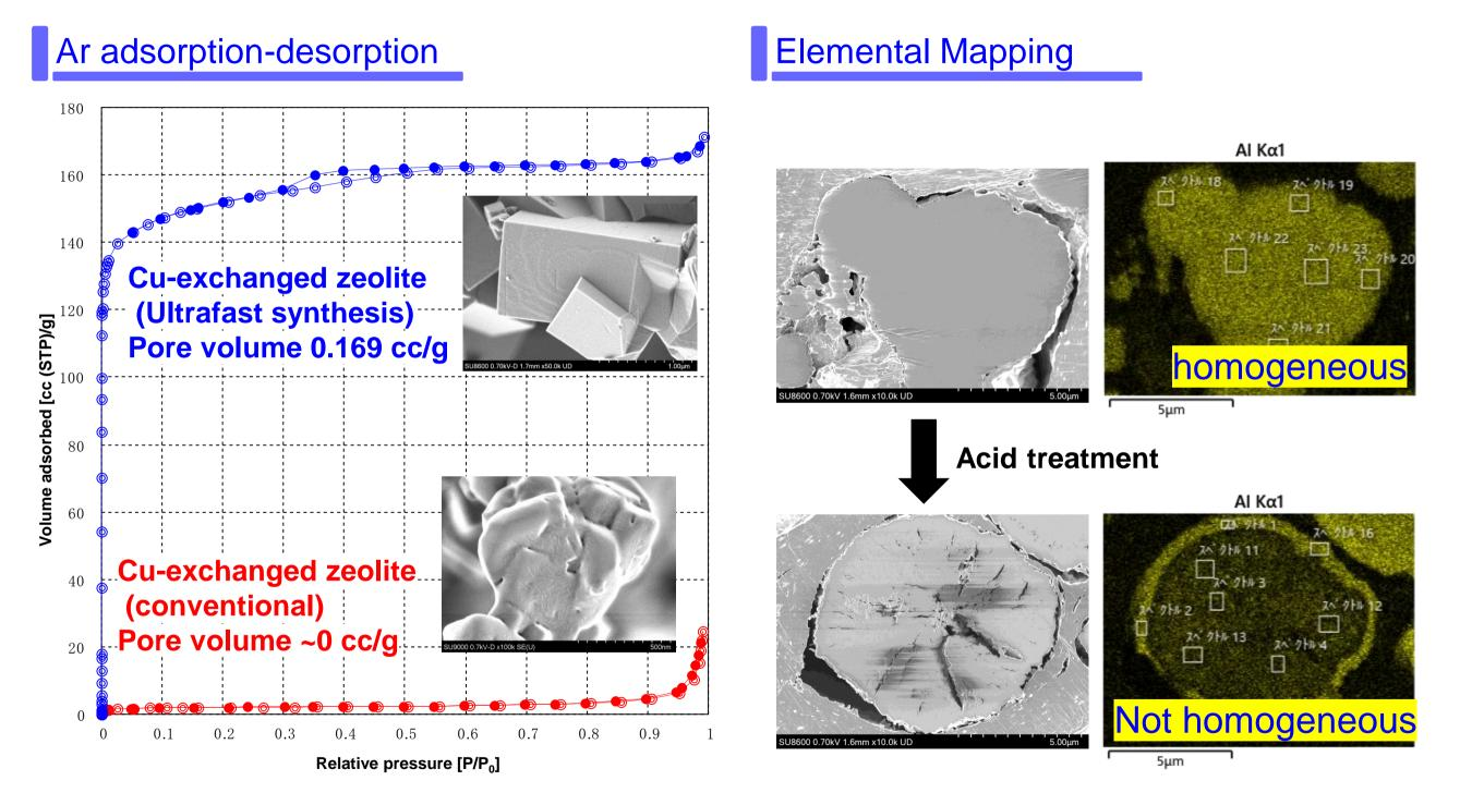
Developed the analysis technique of the degradation and dealumination of zeolite catalyst
