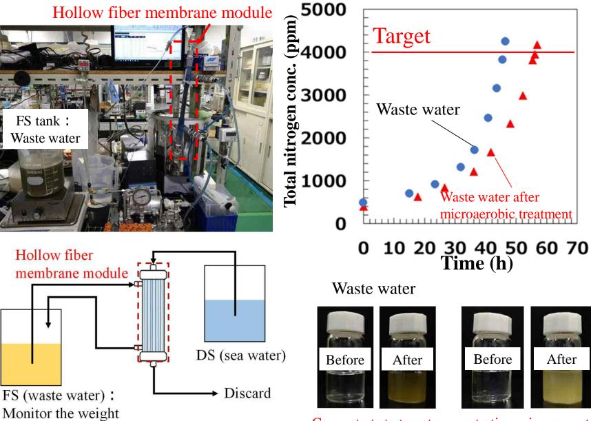
Concentrate to target concentration using seawater
