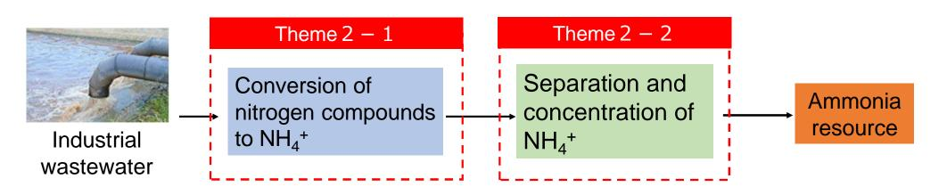
Microaerobic conversion process from nitrogen compounds to NH<sub>4</sub><sup>+</sup>
