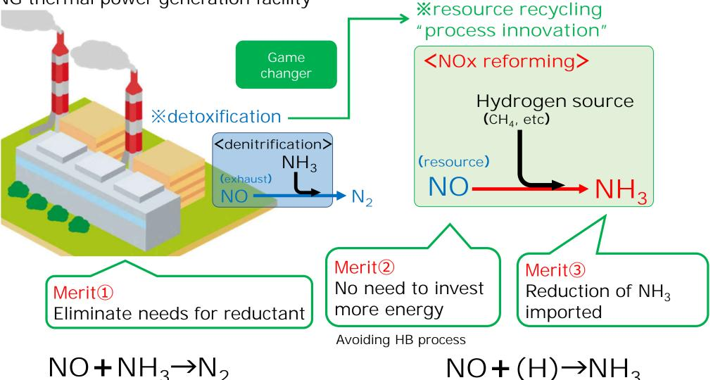
De-NOx utilises  $NH_3$  as it is. Concentration technology for the obtained  $NH_3$  is also developed for other applications.
