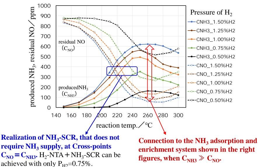
Standard reaction conditions (an atmospheric fixed bed flow reactor) : catalyst W02(0.3mL), total gas flow rate 100 mL/min (space velocity  $SV=30,000 h^{-1}$ ), 0.1% NO, 1.5% H<sub>2</sub>, 0% O<sub>2</sub>, 10% H<sub>2</sub>O, N<sub>2</sub> balance.
