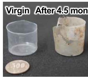
Above: The material before and after 4.5 months in deep-sea. Right: News site reporting the results of the material developed in this project and demonstrating on-site biodegradability.
