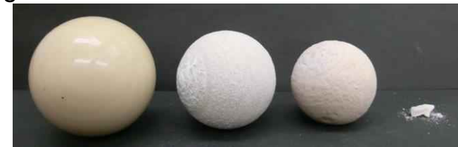
Degradation of PGA ball
