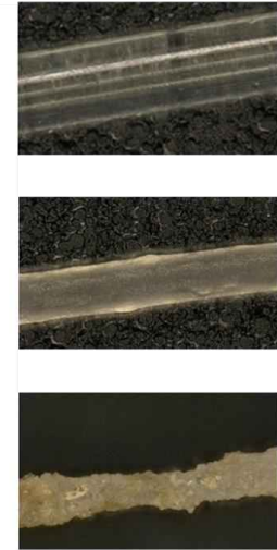
<Degradation Test of the Developed Fiber in Laboratory > Seawater and sediment were collected from the Pacific Ocean (Fukushima pref.).
