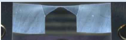
Photograph of tearing PET film just before break
