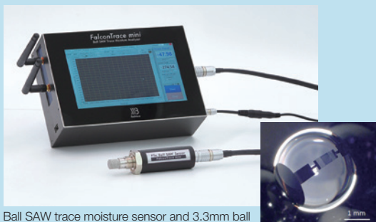
Ball SAW trace moisture sensor and 3.3mm ball SAW element
