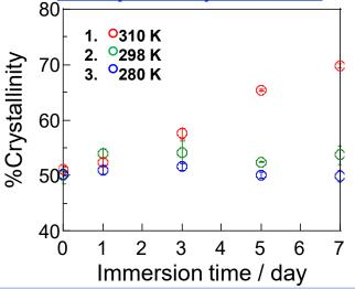
The degradation of the PGA-NF proceeded well when the test temperature was higher than  $T_{g\alpha}$ , however, it was suppressed as the test temperature was equal to or lower than  $T_{g\alpha}$ . In addition, it was found that the degradation proceeded from the amorphous region.
