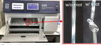
Fishing lines were UV aged by an accelerated weathering machine with total irradiance ca. 300 MJ/m<sup>2</sup> (300-400nm), which is equal to 1 year's irradiation in Choshi. Fibers with knot were employed to simulate the degradation of fishing nets.
