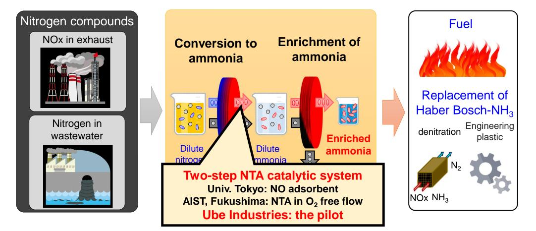
Target of Theme 1 for FY2029 : NOx to Ammonia (NTA) reaction at 50% yield, and complete detoxification of exhaust gas
