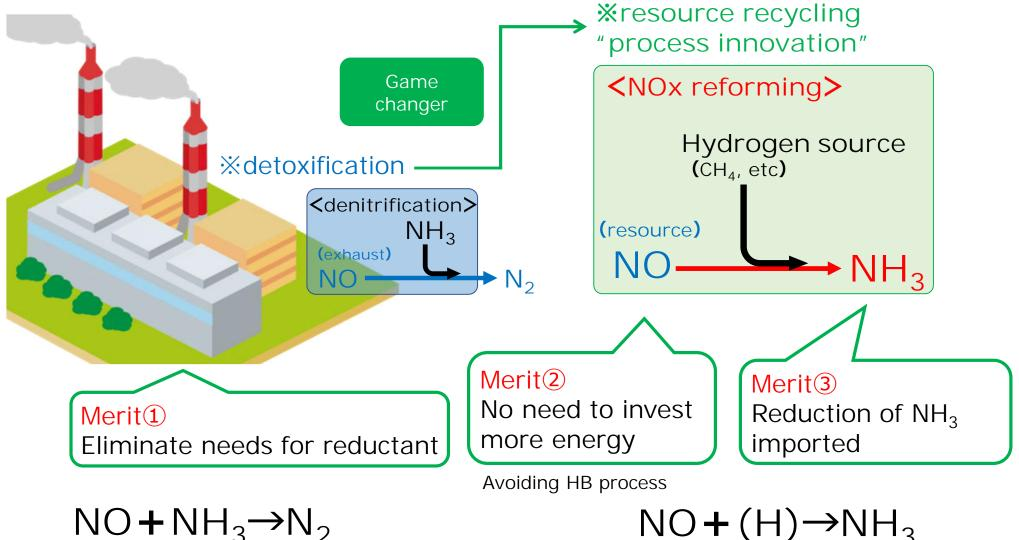
New Energy and Industrial Technology Development Organization: NEDO FY2019 Feasibility Study Program on Energy and New Environmental Technology [Development of ammonia production process from NOx emitted from combustion process]
