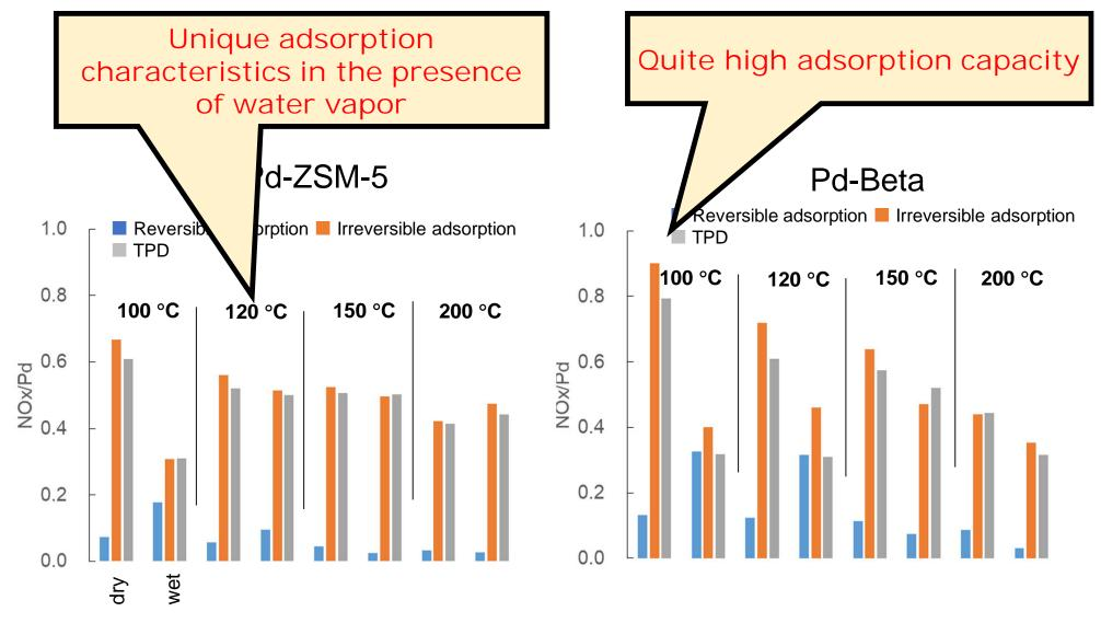
adsorption: NO 500ppm, O<sub>2</sub> 10%, (wet H<sub>2</sub>O 5%)/N<sub>2</sub> 200 mL/min at 100-200 °C TPD: O<sub>2</sub> 10%/N<sub>2</sub> 200 mL/min, heated to 500 °C (10K/min)
