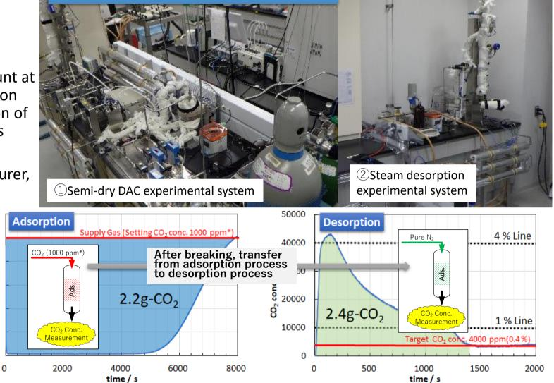
\* 1000 ppm : Indoor CO<sub>2</sub> concentration upper limit standard value based on Japanese regulation. Ex.) CO<sub>2</sub> concentration range : 400 ppm (No occupancy)  $\sim$  1000 ppm (Full occupancy)
