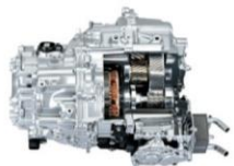
eAxle Offset Design (150kw)
