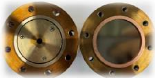
V-type; 60 mmφ, 28 cm 2 -appearance Pd-25Ag sputtered
