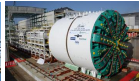
Shield Tunneling Machine
