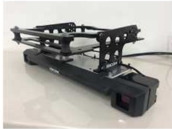
Silent blocks are used to mitigate vibration
