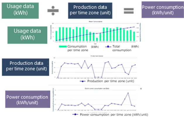
Figure 17 Visualization of power consumption by factory-mounted FEMS
