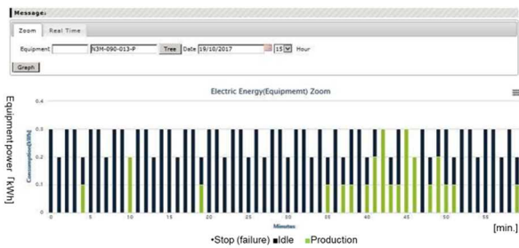
Figure 18 Visualization of operation status of equipment by time zone
