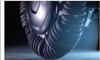
WHILL proprietary front omni-wheel
