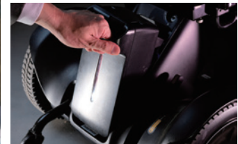
The small, lightweight, user-replaceable lithium-ion battery developed for Model C
