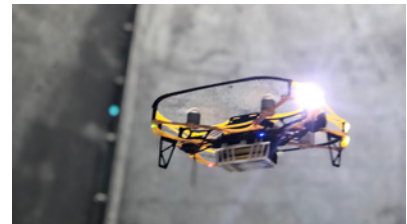
IBIS, a small industrial drone for indoor uses
