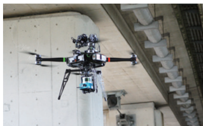
Drone in automatic flight under conditions where GPS is not available
