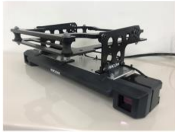
Silent blocks are used to mitigate vibration
