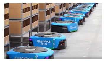
Figure 1.4 The AGVs move customers' orders around the Alibaba's warehouse [5]
