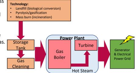
Flowchart of the Biogas Production Process
