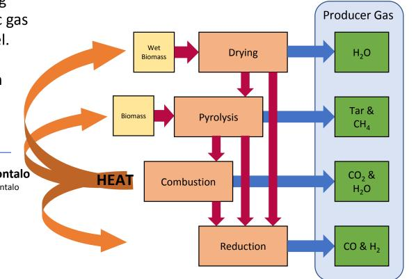
Schematic representation of biomass gasification
