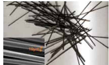
Short fibers for reinforcing concrete made from coal ash and magnified image of its long fibers (Courtesy of Nippon Fiber Corporation KK)
