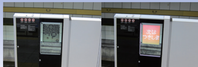
A transparent display installed on the fall prevention barrier at Tokyo Metro Toyosu Station. Left: Transparent mode. Right: Color mode. (Data provided by Sharp Display Technology Corporation)
