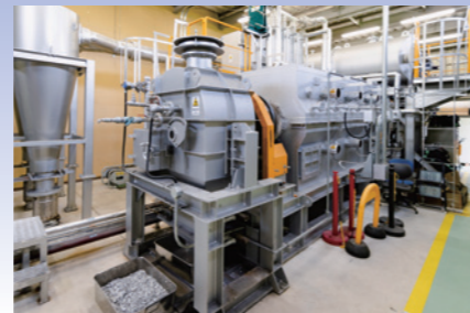
Pyrolysis furnace that separates aluminum mixed with plastic into plastic and aluminum (dry-distillation-type aluminum recovery system)
