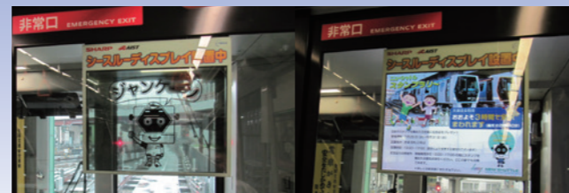
A transparent display installed on the window glass of the driver's cab door on a Saitama New Urban Transit train. Left: Transparent mode. Right: Color mode. (Data provided by Sharp Display Technology Corporation)
