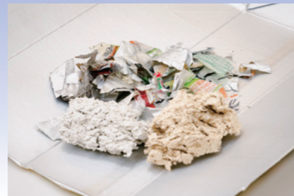
Paper pulp and aluminum mixed with plastic separated and recovered by the pulper separator
