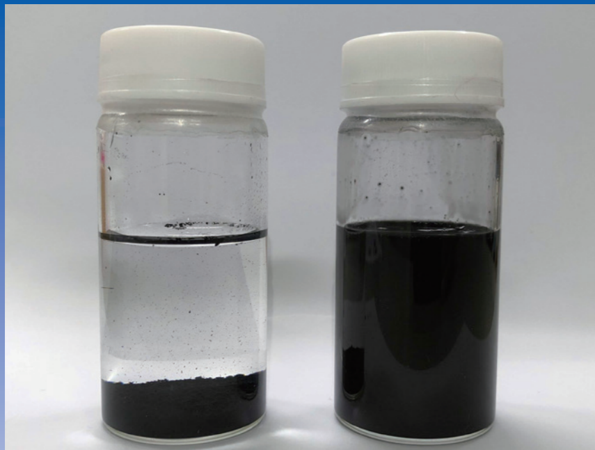
Right: CNTs having disentanglement and dispersion treatment. Left: CNTs with no disentanglement and dispersion treatment. Differences in sedimentation are evident. (Data provided by GSI Creos Corporation)
