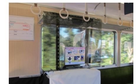
The transparent display was installed on the windows of trains running on a test track owned by Mitsubishi Heavy Industries, Ltd. In this verification, a non-transparent film was hung to verify the case in which a transparent display is used on smoked glass. (Data provided by Sharp Display Technology Corporation)
