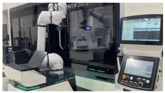
A multi-skilled self-propelled robot with processing assist function
