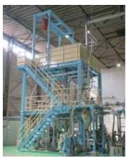
CNF-reinforced resin kneading extruder
