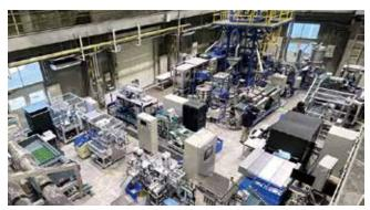
Automatic sorting system for metal resources contained in WEEE
