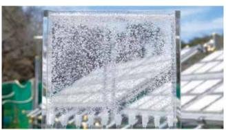
Gas mixture of hydrogen and oxygen generated from photocatalytic panel reactor
