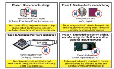
Conceptual diagram of the semiconductor/electronic device life cycle and the technologies to be strengthened
