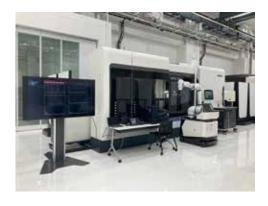
production equipment by combining cloud-based wireless cooperative control platform between automatic guided vehicle with robots (AGV) and production facilities with processing assist module adapted to existing production equipment through local 5G of a high-speed communication standard.
