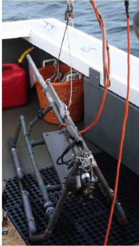
Figure 2. Simrad OE9030/9031 Diver Television System
