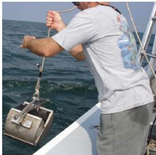
Figure 3. Deployment of VanVeen Grab from the deck of the observation platform
