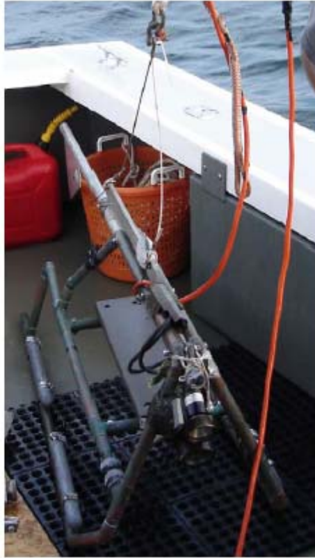
Figure 2. Simrad OE9030/9031 Diver Television System
