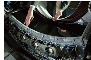
The 320 detector rows have considerable width as a CT system.
