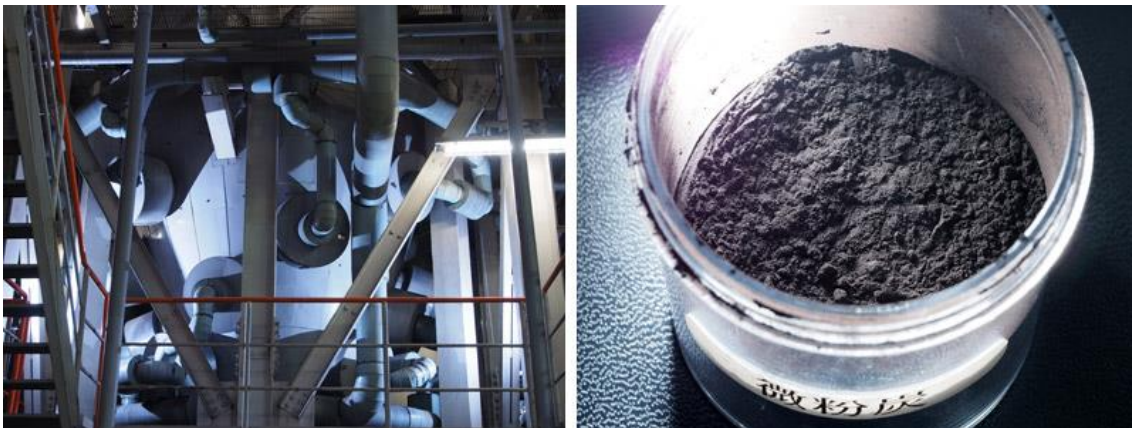
Pulverized coal hopper at IGCC plant of Nakoso Power Plant (left) and use of pulverized coal as fuel (right)
