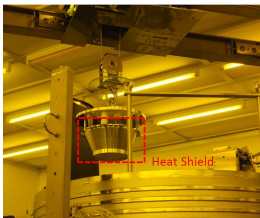
図Ⅲ. 2. 2. 4-4-8 HSFET本体へ搬入中のHeat Shield
