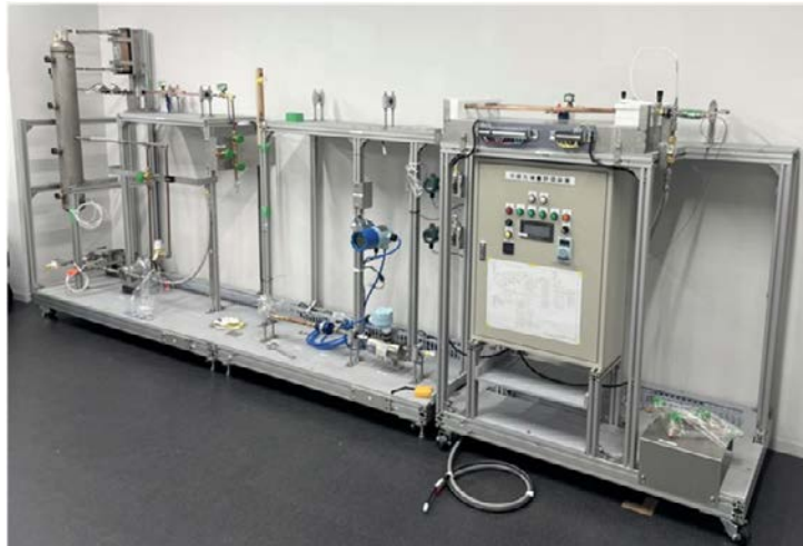
External view of refrigerant charge evaluation system
