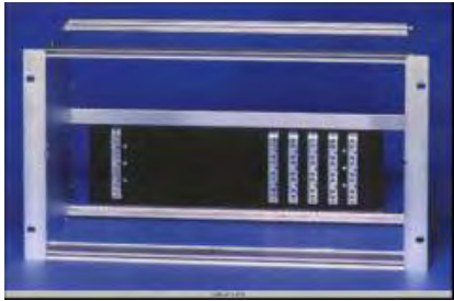
Optical backplane mounted in 19-inch rack
