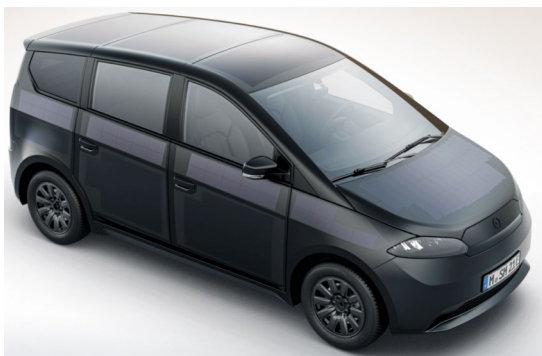
Fig. 1.1-1 Example of a PV-powered Vehicle (1) Sono Motors - Sion 9
