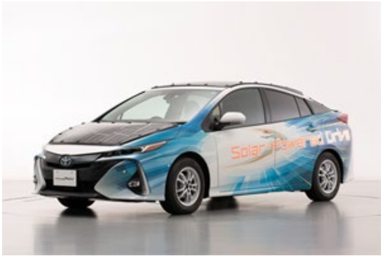
Fig. 1.2-1 PV-powered demonstration vehicle (1) Prius PHEV (Toyota Motor Corporation) 24
