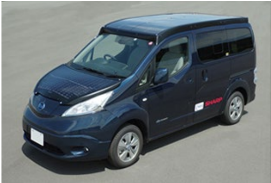
Fig. 1.2-2 PV-powered demonstration vehicle (2) eNV200 (Nissan Motor Co., Ltd.) 25
