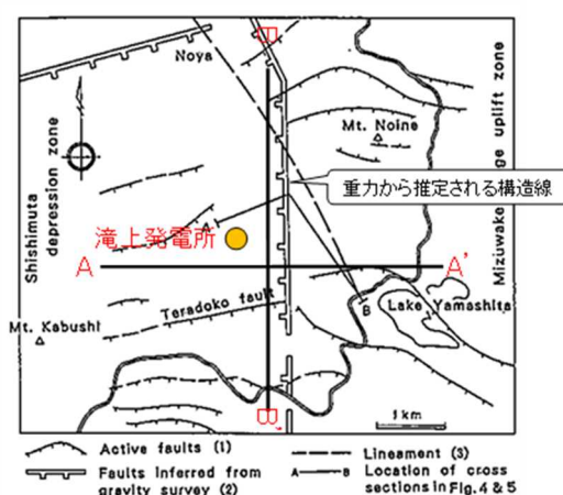
Fig. 7.3.1 NS fault suggested by gravity data (modified from Takenaka et al. , 1995). The yellow circle shows the TP-2 wellhead and the geothermal powerplant location. The geological section A-A and B-B is shown in Fig. 7.3.2.
