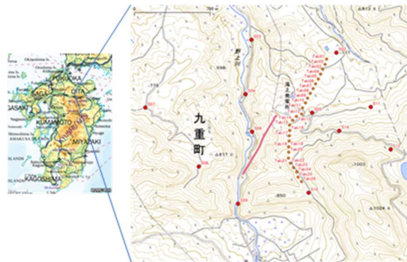
Fig. 7.3.3 Location map of TP-2 geothermal well (red line), seismic sources (red stars) and surface geophones (yellow dots).
