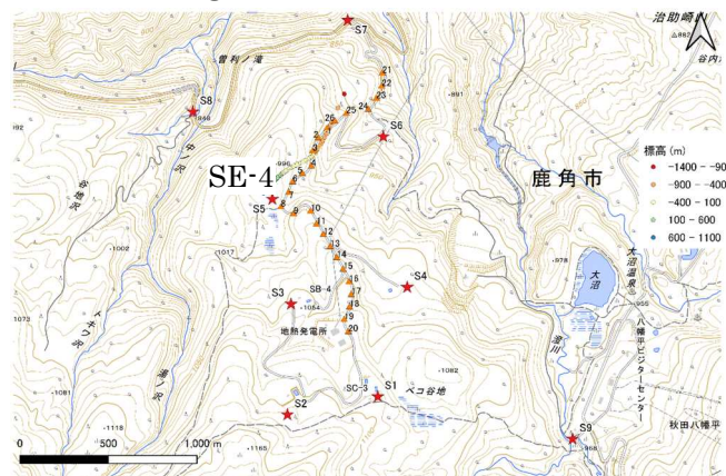
Fig. 7.2.3 Location map of the Sumikawa study. Stars are seismic source locations. The SE-4 is a geothermal well. Triangles are surface geophones.
