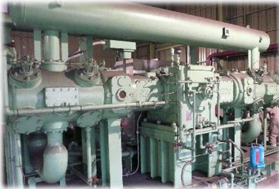
Reference image: Horizontally opposed type compressor
