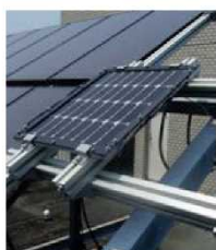
PV module using 3J tandem cell Area: 983 cm 2 STC: 31.17% 2016/08 - up to now
