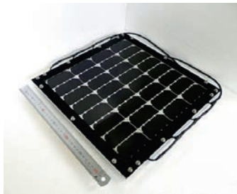
Module by Sharp Corporation Conversion efficiency: 31.17% (968 cm 2 )
