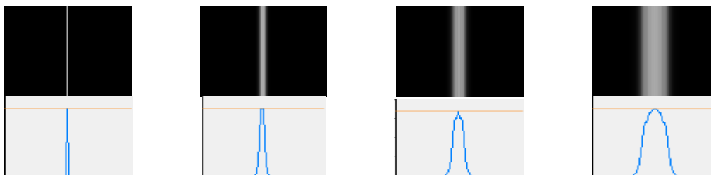
a) defocus 0 \mu m b) defocus 10 \mu m c) defocus 20 \mu m d) defocus 40 \mu m
