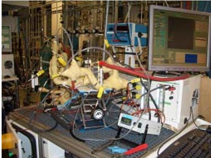
Polarization curve test in HNEI
