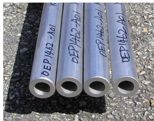
図Ⅲ.2.3(2)2-9 鋼管材の外観 (34.0 φ × 6.5t)
